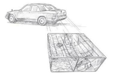
The modified fuel tank is only partially filled with gas and contains a cavity to conceal a person being exfiltrated from a hostile area. From the outside, the car appears normal. Phil Franke
