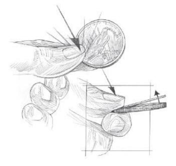
Squeezing a spot near the edge of the coin caused it to open. Phil Franke
