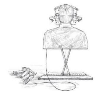
The JIB had a trigger grip to rotate the head and a collapsing scissor mechanism for
