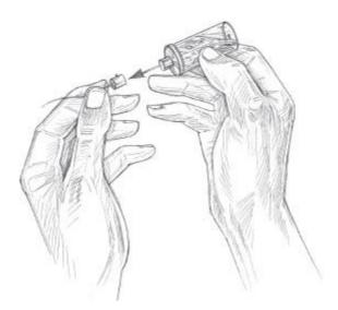
Rigid container showing stopper at top to which thread is attached. Stopper closes top air vent. Exit hole is in center of bottom of container. Phil Franke
