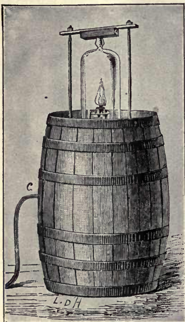
FIG. 8.—Boutan's apparatus for using a magnesium flash-light under water. The reservoir for the magnesium powder, the rubber bulb, and the weights used to steady the apparatus are not shown in the figure. (Copy of fig. 3 in Boutan, 1893.)
