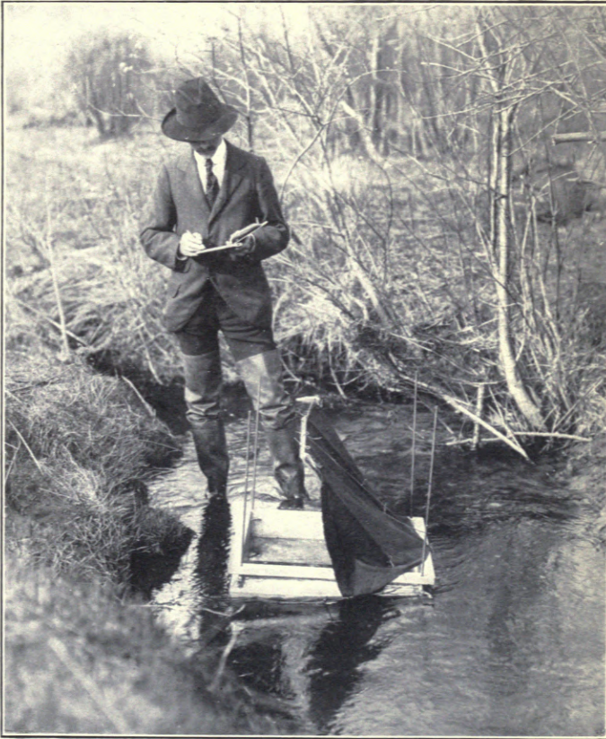
FIG. 2. TWO-FOOT WATER GLASS SUPPORTED ON FOUR LEGS AND PROVIDED WITH SCREEN, AS USED FOR STUDYING AND PHOTOGRAPHING LAMPREYS ( LAMPETRA WILDERI ).
